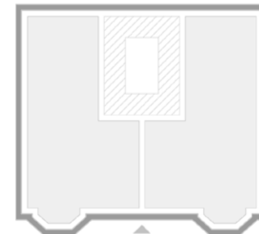
Block Eight: Two Flats Rear Open Staircase Bay Windows
