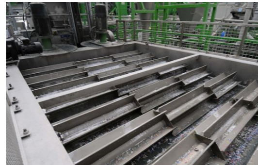
Plastic separation by flotation Allows heavier contaminant to sink to the bottom to be discarded or to separate the heavier PET from the lighter PP/PE
