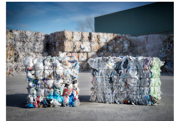
Baling: 72 hour quarantine for material upon arrival. Materials are sorted by categories and amalgamated before being sent to processors.
