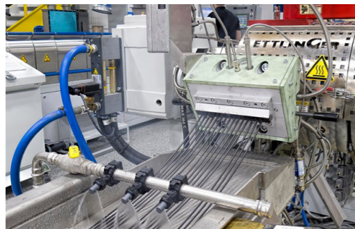
Melting and Extruding The material is melted and extruded into fine even strands.
