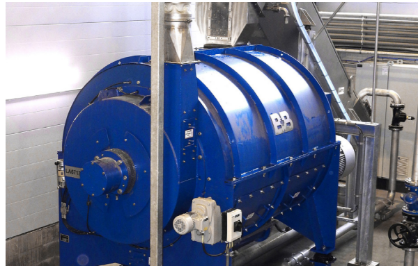
De- Watering and Drying The process reduces traces of moisture on the material to nominal figures.
