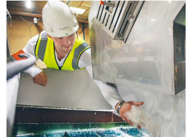
Washing and shredding Materials are decontaminated by washing (type of washing depending on plastic and contamination) then split in smaller fibres / particles for use in production lines or melting.
